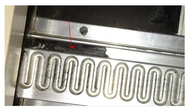
Here is the track where the bearing block was binding on the track and making the popping noise and
