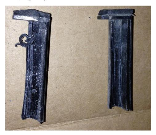
This is a picture of the plastic shoe that was broken inside the front half of front driver slide, you can see how one side was broken off and allowed the metal bearing block to float in the tracks.
