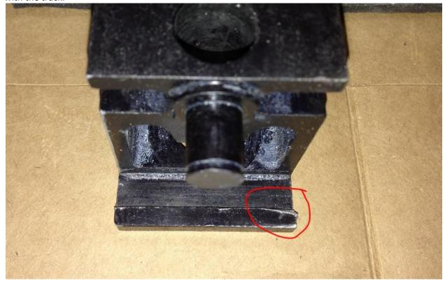
Both of these slide mechanism for the driver side front slide only had 10-15 opening and closings on them before they failed, and this was the second set of slides (the improved ones) and they lasted about the same amount of openings.
