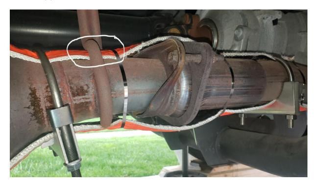
The oxygen sensor is visible at the top.
