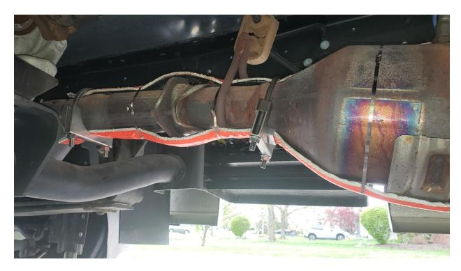
I had to use two of the supplied stainless steel bands to make one long band in order to go all the way around the catalytic converter.
