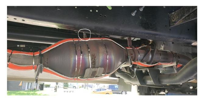
The rear clamps are on a bit of an angle because the CatStrap runs to one side to stay away from the oxygen sensor and also because the opening in the frame that the CatStrap loops through is not inline with the exhaust system.
