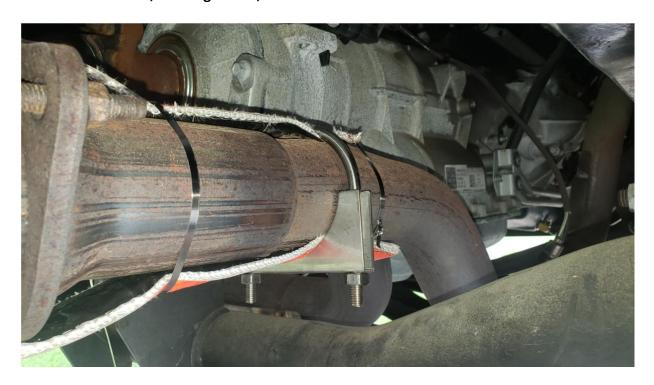
Note on this next picture that I was able to slip the CatStrap underneath the welded mount on the top of the exhaust pipe but not on the bottom.
