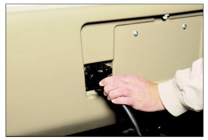
With a seven-pin connector and the supplied pigtail, owners of nearly all 2006 and newer Winnebago Industries motor homes have pre-wired options not only for turn signals and brake lights, but also items such as running lamps, backup lamps, and an electric brake system on the towed unit.
