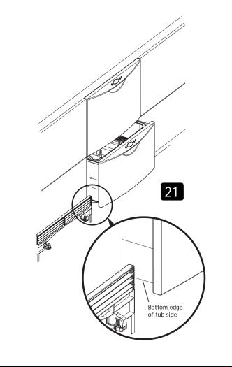
21 Partially open the bottom drawer. Turn Prefinished Toe Kick upside down and hold vertically against the bottom edge of the *Tub side* (not the drawer front).
