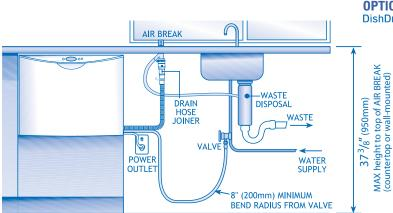
**OPTION 3** DishDrawer<sup>®</sup> using Air Break with Drain Hose Joiner.
