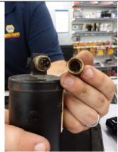
Note the check-valves are used to block descant from contaminating the A/C System in the event the Receiver Dryer fails.
