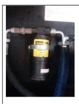
OEM PARKER Receiver-Dryer (Vintage 2003) with HP-Red Schrader port on right. This line comes from your Condenser. **Napa Cross: #218093** (\$34); Freightliner Part # GAFP110704 (\$75). Other crosses include A/C/Delco #17-9969 or Fleetwood# 151779 or RV218396.
