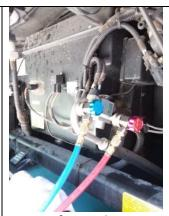
From Left to Right, notice the AC wire connector, the A/C relay, Thermostat, Blue LP Schrader port, Red HP Schrader Port... surrounded by a Binary Switch on the left and a Condenser Fan Control Switch on the right. And in the background that shiny block is your TXV-Expansion Valve. (You should clean all these electrical contacts!)
