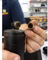
Note the check-valves are used to block descant from contaminating the A/C System in the event the Receiver Dryer fails.
