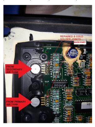
Note: The toughest part of the job was separating the red and green air lines to the VDC.
