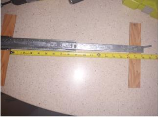
HINT: Before you reuse your old screw holes in the pantry, get some wood toothpicks and hammer toothpicks into the old screw holes before you tighten up the wood screws with your new sliders. I also recommend you add silicone caulk to the back of the pantry slider for added support. The latch is spring loaded and has a locking tab. In the picture this tab is square, but it can get warn down or even breakoff.
