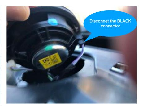
There are two connectors, one on either side of the speaker. One is black, one is white. Disconnect the BACK one only.
