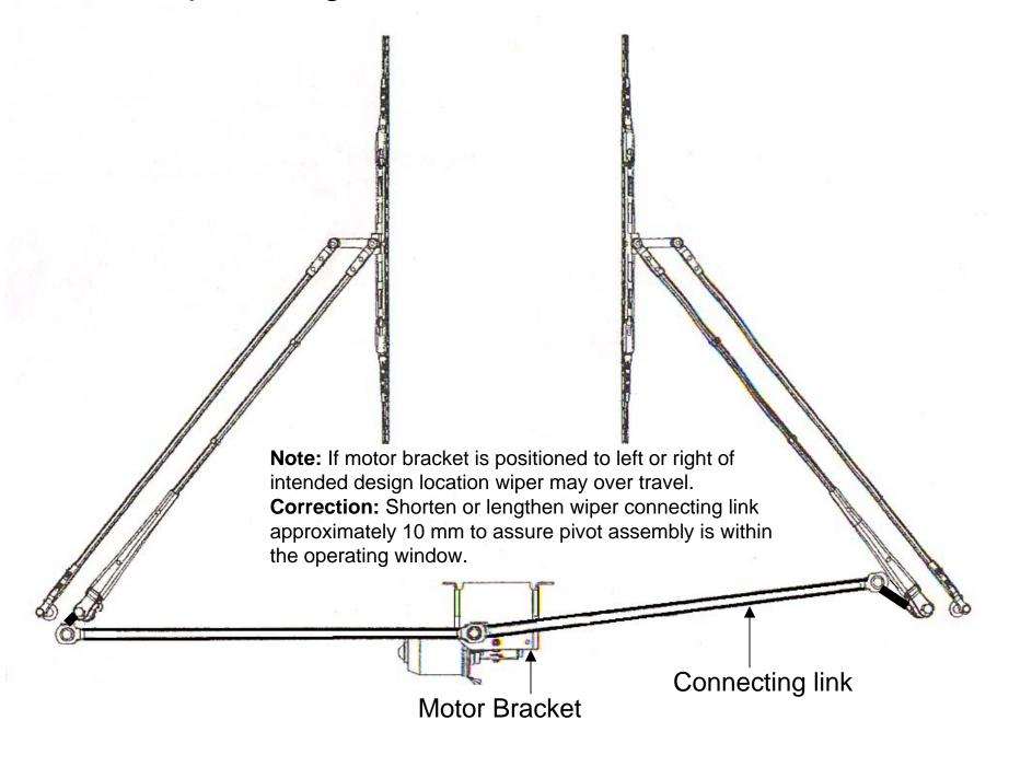
Wiper configuration used with one piece windshield.
