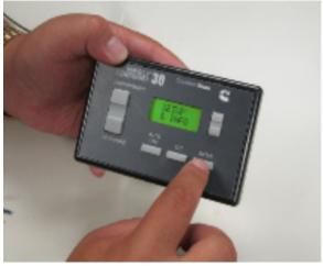
3. Press the 'Up' button 4 times to display the SWV.
