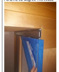
Likewise, all slides need to measure the same distance from the left. (Use painter sticks or other material as shims.) This picture shows 3 slides. The top and bottom are PTO slides from Home Depot and the center slide is the one I got at Winnebago and has a latch.
