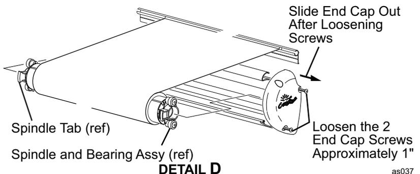
6. Lift the roller tube out of the deflector.
