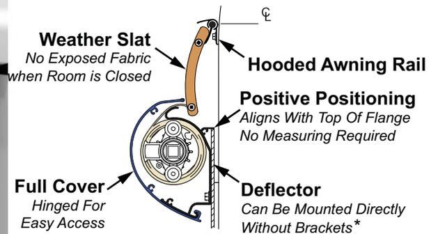
\* An optional mounting bracket is available for curved flange applications or applications that the deflector cannot be mounted directly.
